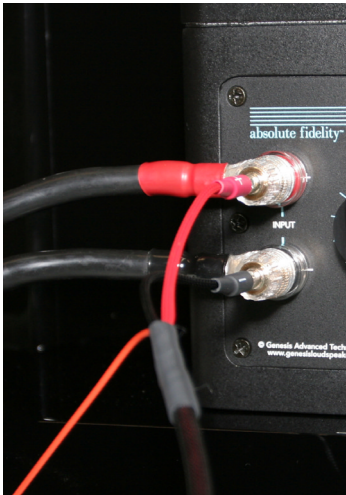
Servo-Bass Interconnects parallels speaker cable inputs
